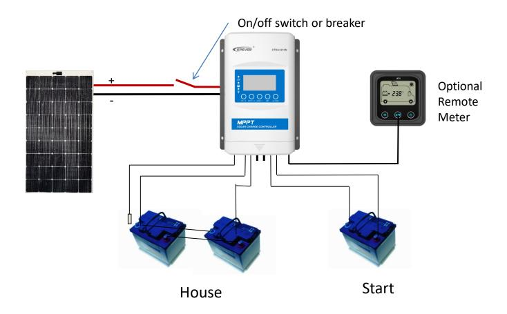
Attach controller to battery banks first and to solar panels second.
