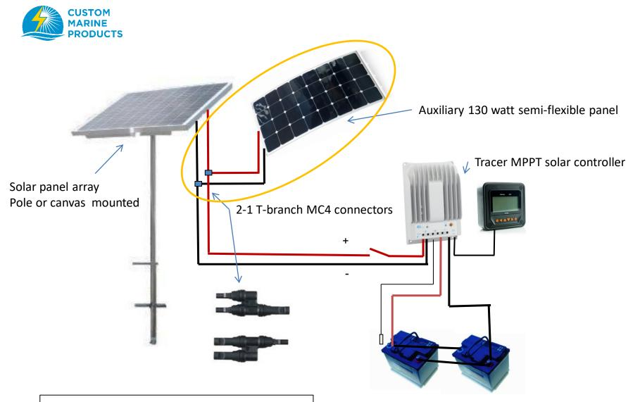
Wiring diagram showing connection of an auxiliary 130 watt solar panel when extra power is needed.
