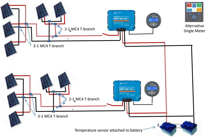
Place a 10 amp fuse in the positive line for each panel at the MC4 T branch.
