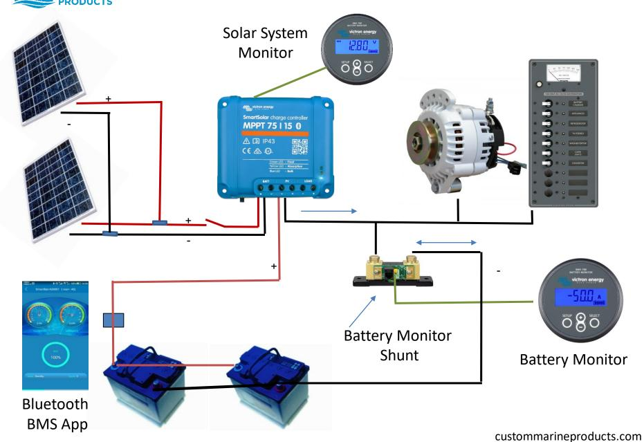
Two Solar Panels Wired in Parallel with a Battery Monitor and MultiPlus Inverter/Charger
